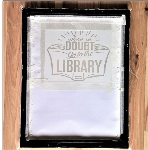
Tape off (masking) exposed areas of the silk screen with masking tape or a combination of masking tape and paper.
